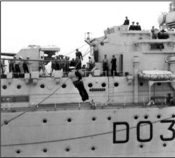
Jackstay transfer between HMS Opossum destroyer HMS Concord
